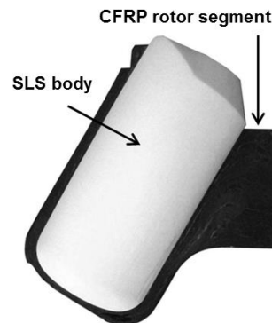
Fig. 3. Selective laser sintered components of a cup recess in a CFRP rotor segment.
