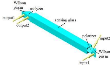
Fig. 3. Dual-input and dual-output sensor.
