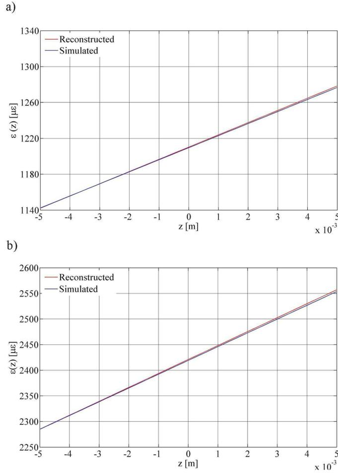
Fig. 3. Simulated strain profile and reconstructed strain profile: a)  $\varepsilon(z) = 1209\mu\varepsilon + (13.44\mu\varepsilon/\text{mm})z$ ;
