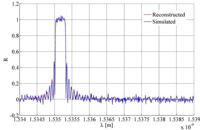
Fig. 2. Simulated reflection spectrum with 2.5% noise and reconstructed reflection spectrum of the grating.
