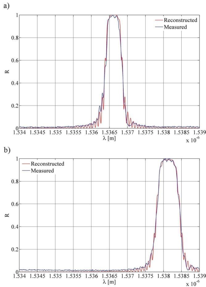
Fig. 7. Measured reflection spectrum and reconstructed reflection spectrum of the grating for strain profile:
