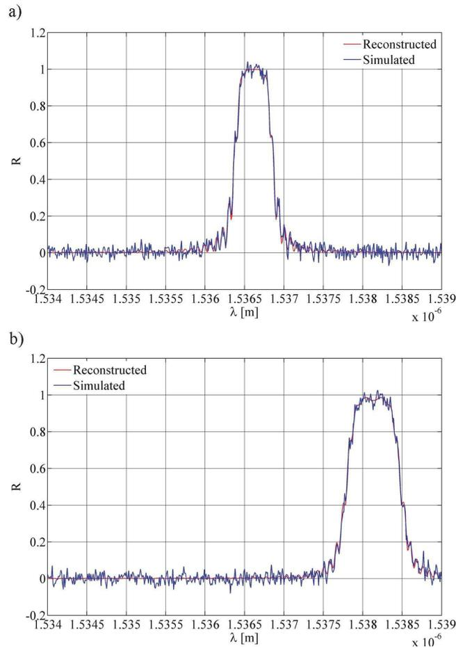
Fig. 4. Simulated reflection spectrum and reconstructed reflection spectrum of the grating for the strain profile: a)  $\varepsilon(z) = 1209\mu\varepsilon + (13.44\mu\varepsilon/\text{mm})z$ ; b)  $\varepsilon(z) = 2419\mu\varepsilon + (26.88\mu\varepsilon/\text{mm})z$ .
