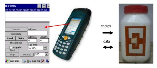
Fig. 6. The visualization of reading of electronic product code during the measurements of MRD.
