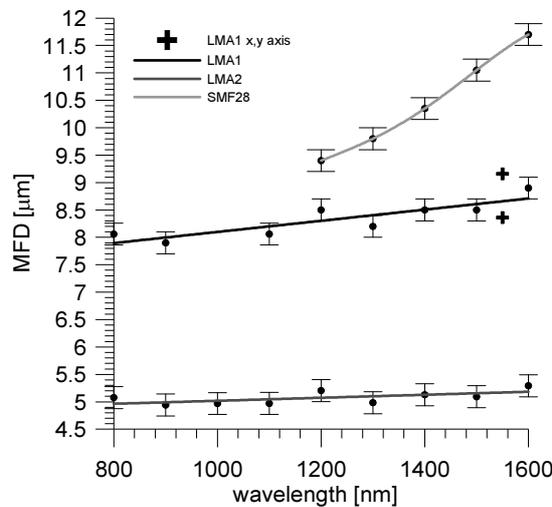
Fig. 9. A plot of the MFD as a function of wavelength for all measured fibers.
