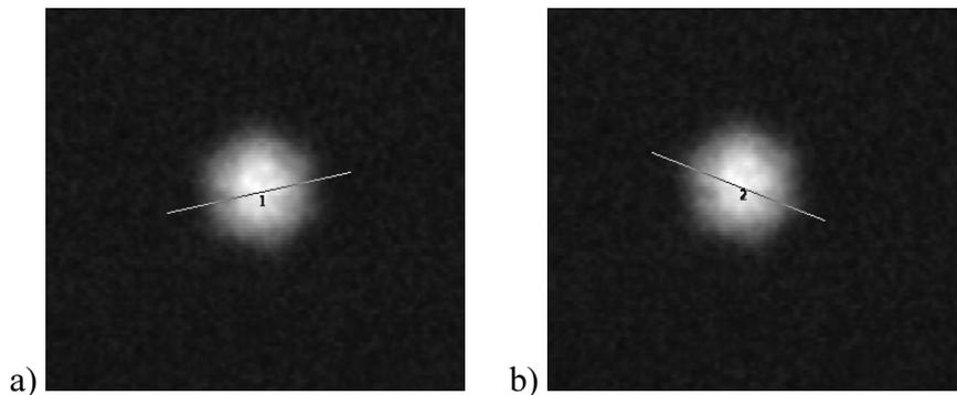
Fig. 6. Near-field images taken using the proposed measurement system: a) the method of determining the minimum diameter and b) the method of determining the maximum diameter.
