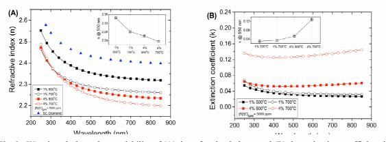
Fig. 3. Wavelength-dependent variability of (A) the refractive index n and (B) the extinction coefficient k in boron-doped diamond films deposited under various conditions related to the methane admixture and the substrate temperature. For comparative purposes, the refractive index measurements for a single-crystal diamond are shown ( $\blacktriangle$ -SCD) [41]. Insets: the variability of n and k measured at 550 nm.
