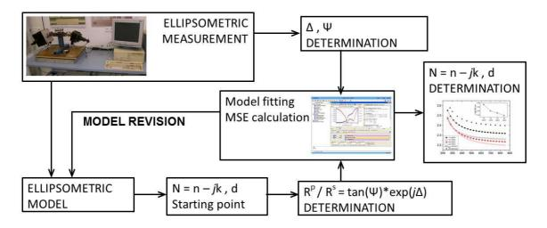
Fig. 1. The scheme of the ellipsometric measurement algorithm.
