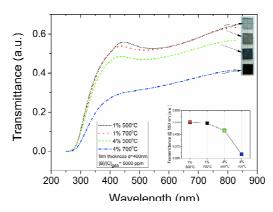
Fig. 4. The transmittance of boron-doped diamond films deposited on transparent quartz substrates under various conditions related to the methane admixture and the substrate temperature. The film thickness for each sample is also given. Inset: the variability of transmittance measured at 550 nm and photos of the presented BDD samples.
