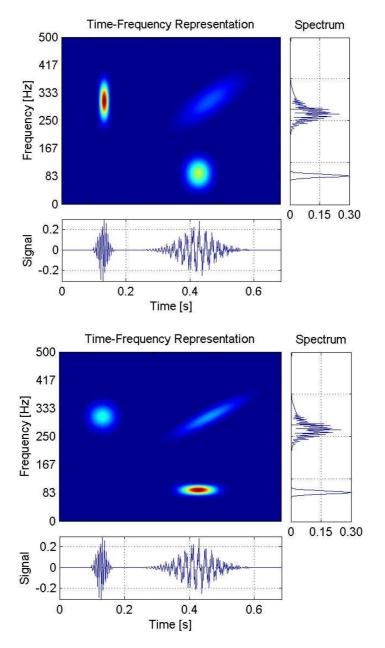
Fig. 2. A practical example of the STFT decomposition for a narrow time window (top part: Hanning, 32 samples) and a wide time window (bottom part: Hanning, 128 samples).
