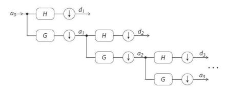
Fig. 8. A wavelet decomposition tree:  $a_0$  - the original signal,  $d_i$  – the detail in the i-th scale,  $a_i$  – the approximation in the i-th scale.
