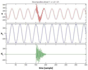
Fig. 9. The effect of a one-level wavelet decomposition.
