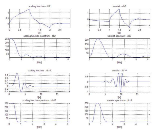
Fig. 11. Two examples of wavelets with scaling functions and their spectra (2<sup>nd</sup> order Daubechies – db2, 10<sup>th</sup> order Daubechies – db10).
