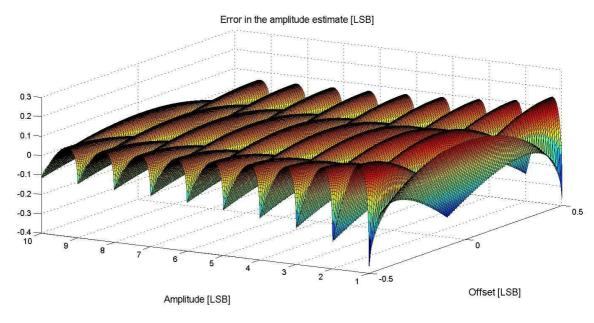
Fig. 2. The estimation error of the sine wave amplitude after the quantization as a function of the amplitude and the offset.
