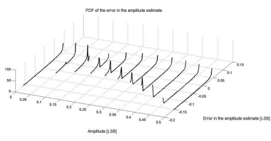
Fig. 5. The behavior of the PDF of the error in the amplitude estimate for different sine wave amplitude values.
