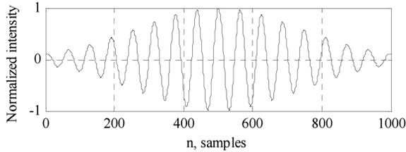
Fig. 4. The representation of 1D line of WLI.
