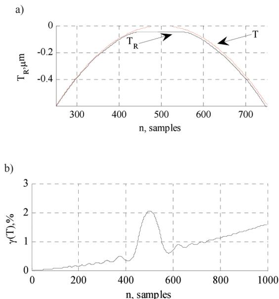
Fig. 9. The results of spherical surface reconstruction: a) the shape of the profile of the simulated surface (curve  $T$ ) and the reconstructed surface (curve  $T_R$ ); b) the reconstruction error graph.
