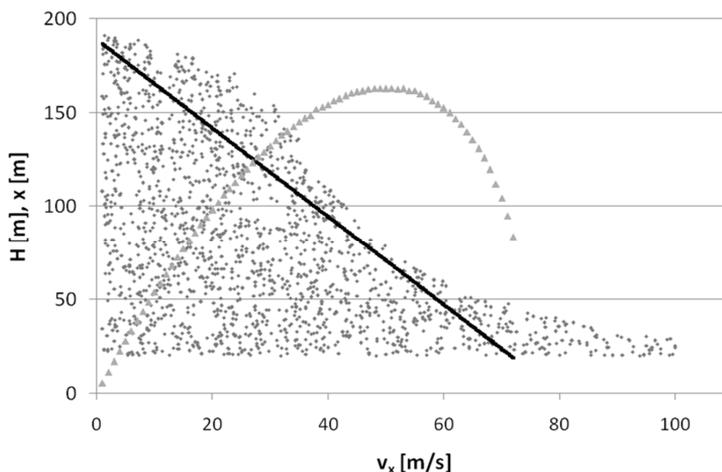
Fig. 6. A cloud of points fulfilling the accuracy criterion of the capsule airdrop system (light-grey diamonds), the straight line described by (14) (black line), and the dependence of the airdrop range on the flight velocity (as well as the corresponding height of the release point) at the moment of airbag release for the points described by (14).
