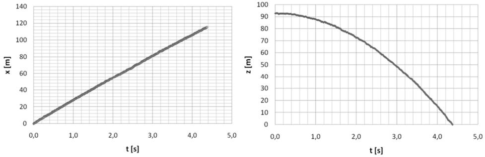
Fig. 4. Dependence on time of the capsule's horizontal and vertical coordinates.
