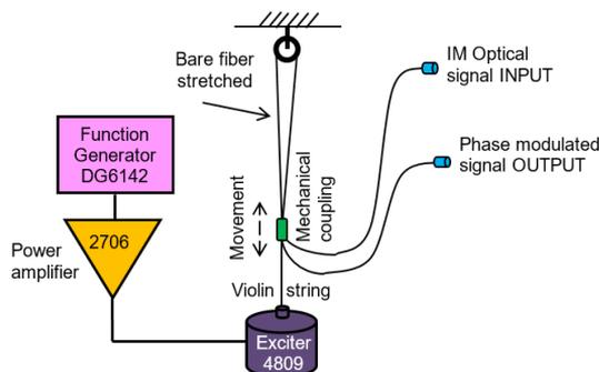
Fig. 2. A block diagram of the fibre stretcher.
