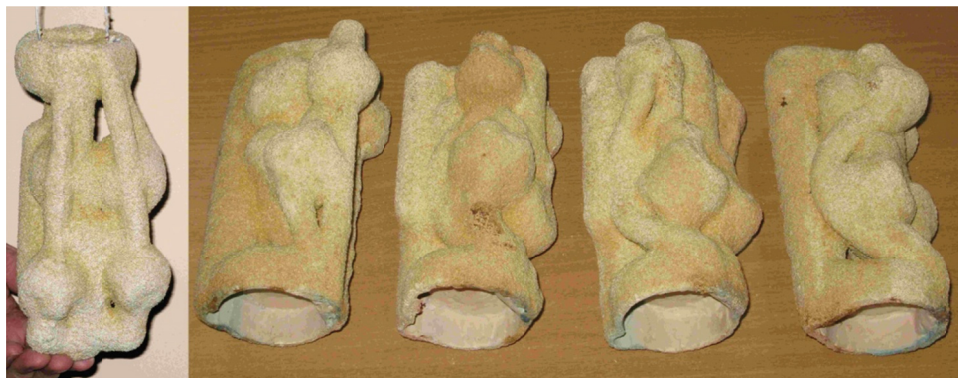
Fig. 30. Raw ceramic moulds before and after de-waxing
