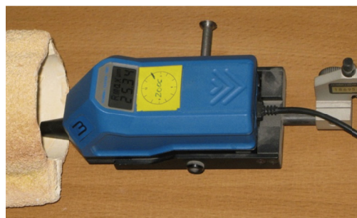
Fig. 31. Measurement of the ceramic mould surface roughness using a Hommel Tester T500 device
