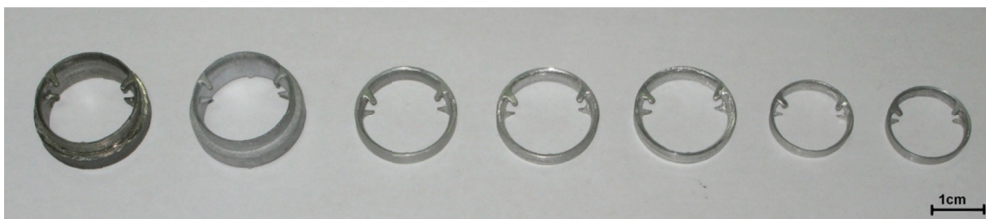
Fig. 26. Different designs of the heart valve castings
