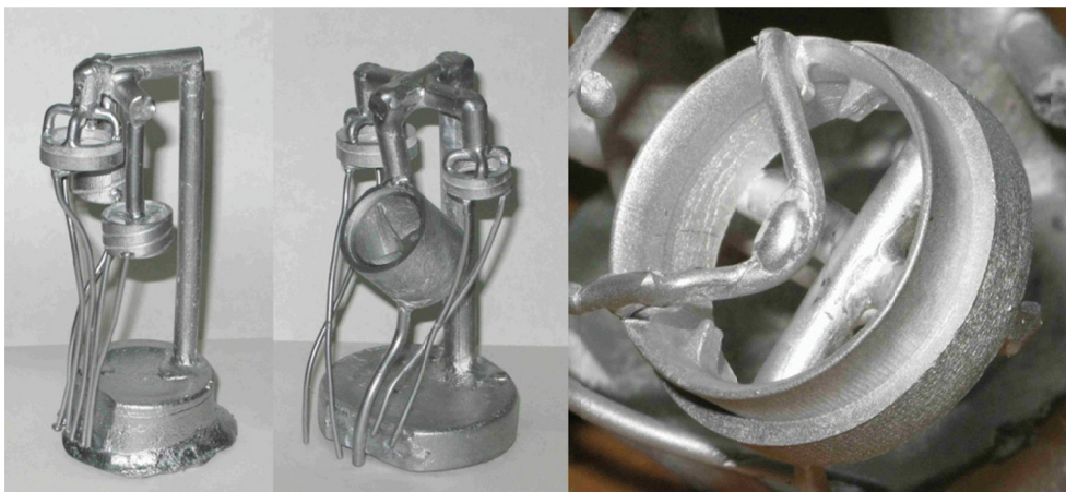
Fig. 25. Experimental castings of the heart valve made from an AlSi7Mg alloy
