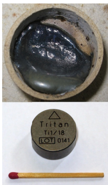
Fig. 21. Titanium before and after remelting in the experimental ZrO 2 crucible and the results of chemical analysis of the titanium feedstock and metal remelted in the crucible using Niton XL3t spectrometer
