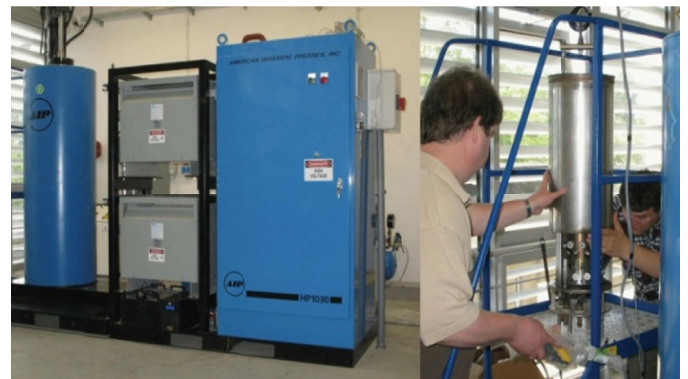
Fig. 36. The device for hot isostatic pressing of castings – HIP
