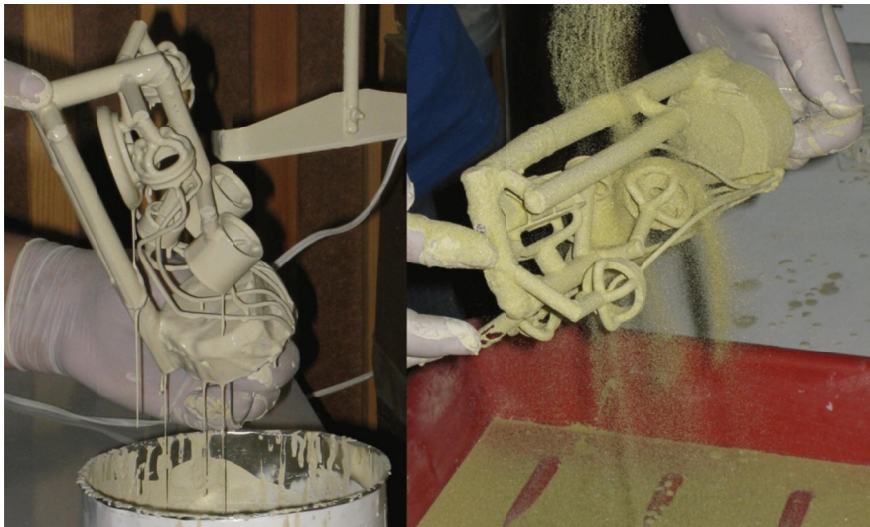
Fig. 28. Successive steps in the process of making the first layer of a ceramic mould (castings of the heart valve and hydraulic drive unit components)
