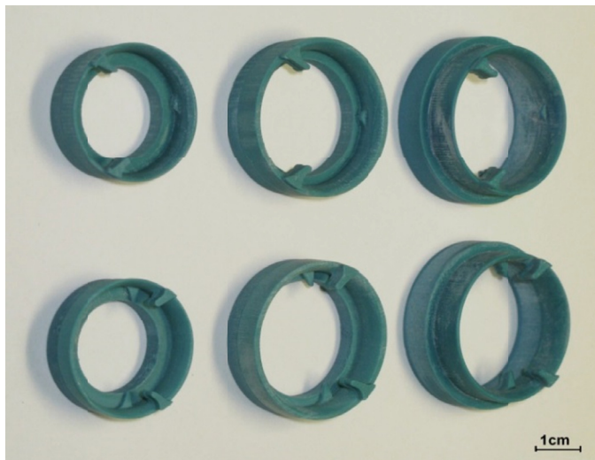
Fig. 12. Different versions of the heart valve rings obtained from a DodJet printer
