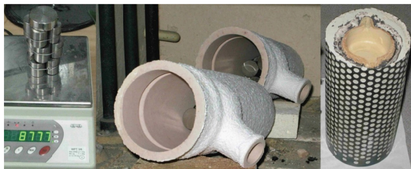
Fig. 33. Weighing of titanium feedstock, drying of crucible with feedstock placed inside, and ceramic mould ready for pouring with molten metal
