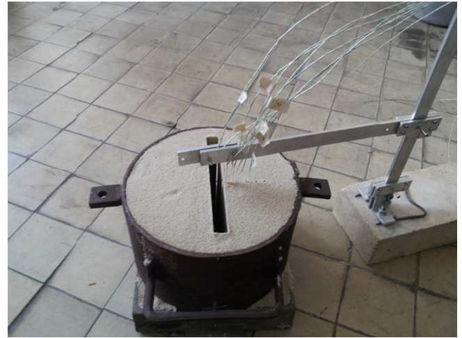
Fig. 2. The experimental mould before pouring. Visible thermocouples mounted in the mould cavity and in the mould body
