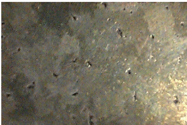
Fig. 2. Visible porosity cavities on surfaces of samples
