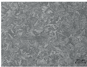
Fig. 9. Microstructure of S460 steel, bainite + martensite ( v_H=100 K/s i v_{8/5} = 100 K/s)
