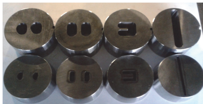
Fig. 6. The dies and backers (above) for extrusion of solid sections
