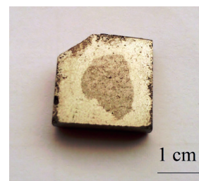
Fig. 3. Macrostructure of the sample during disproportionation reaction
