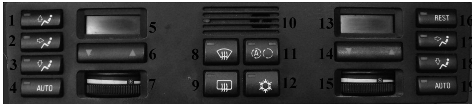
Fig. 2. Control panel for the heating and air – conditioning system installed in BMW cars (1994-2001) 1- air supply to windscreen / panes; 2 - air supply to the head (driver's side); 3 - air supply to the feet (driver's side); 4 – air – conditioning automatic control (driver's side); 5 – temperature indicator (driver's side); 6 – temperature control (driver's side); 7 – air supply intensity (driver's side); 8 – defrosting function; 9 – rear pane heating; 10 – vehicle inner temperature sensor; 11 – closed loop air cycle; 12 - air – conditioning ON; 13 – temperature indicator (passenger's side); 14 – temperature control (passenger's side); 15 – air supply intensity (passenger's side); 16 – residual heat utilization; 17 - air supply to the head (passenger's side); 18 - air supply to the feet (passenger's side); 19 – air – conditioning automatic control (passenger's side);
