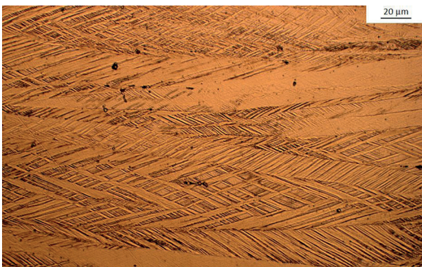
Fig. 1. Structure of high manganese austenitic X73MnSiAlNbTi25-1-3 TWIP-type steel with mechanical twins and slip bands in both systems obtained after tensile test in static conditions
