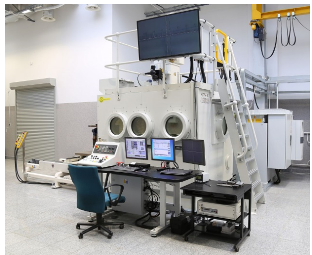
Fig. 1. The electron beam machine for welding and surface modification model XW150:30/756
