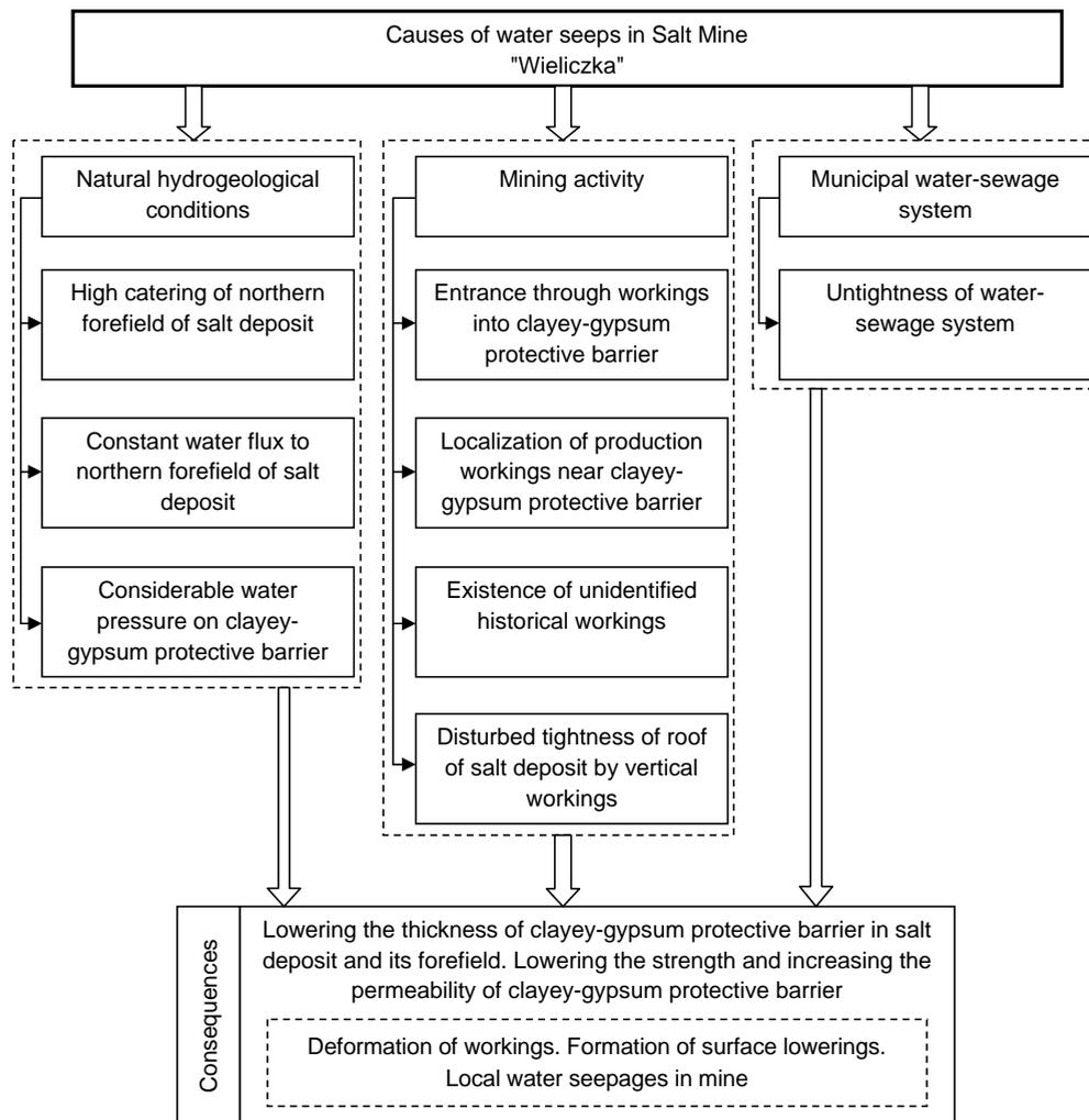
Fig. 2. Block diagram illustrating causes of water fluxes in the Salt Mine "Wieliczka"
