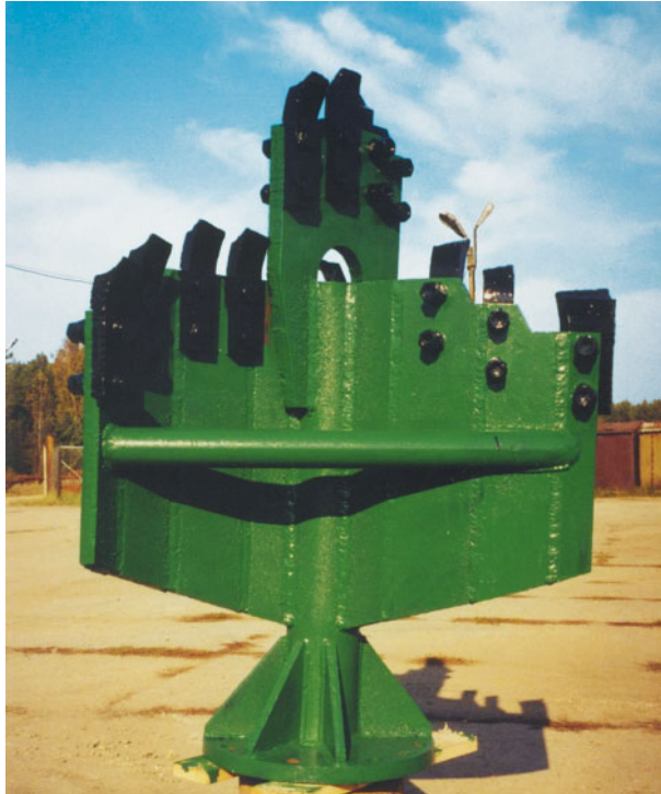
Fig. 1. Large-diameter cutter bit with profiled wings \varnothing 1.16 m
