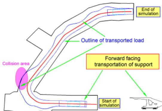
Fig. 14. Exemplary simulation. Determination of outline of transported load. Forward facing transportation of the support
