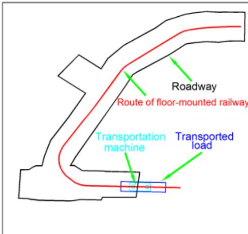
Fig. 10. Components of simulation model
