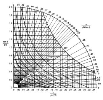
Fig. 6. Circular failure chart [8]
