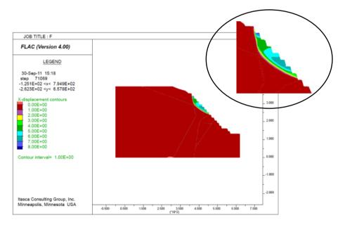
Fig. 3. X-displacement contours in studied section by FLAC software
