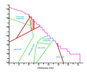
Fig. 8. Geological cross-section of Chadormalu iron open pit mine southern wall
