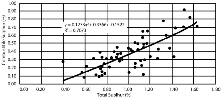
Fig. 2. Relation between total and combustible sulfur (Haxhiu, 2004)
