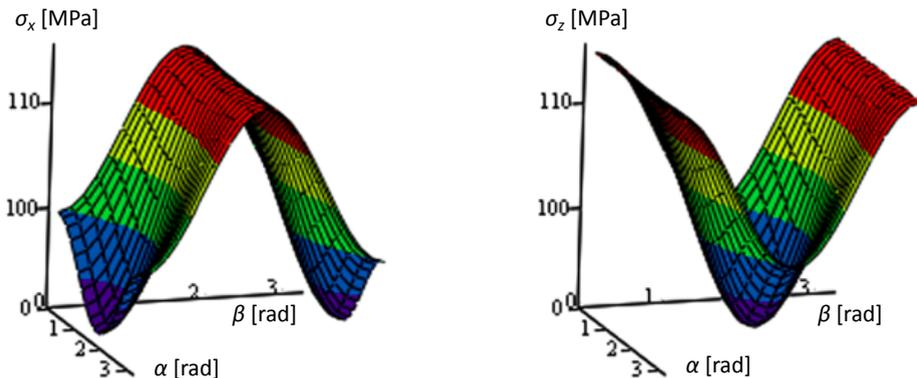
Fig. 1. Transformed in-situ Stress vs. Wellbore Inclination and Azimuth, Graph in Cartesian Co-ordinate
