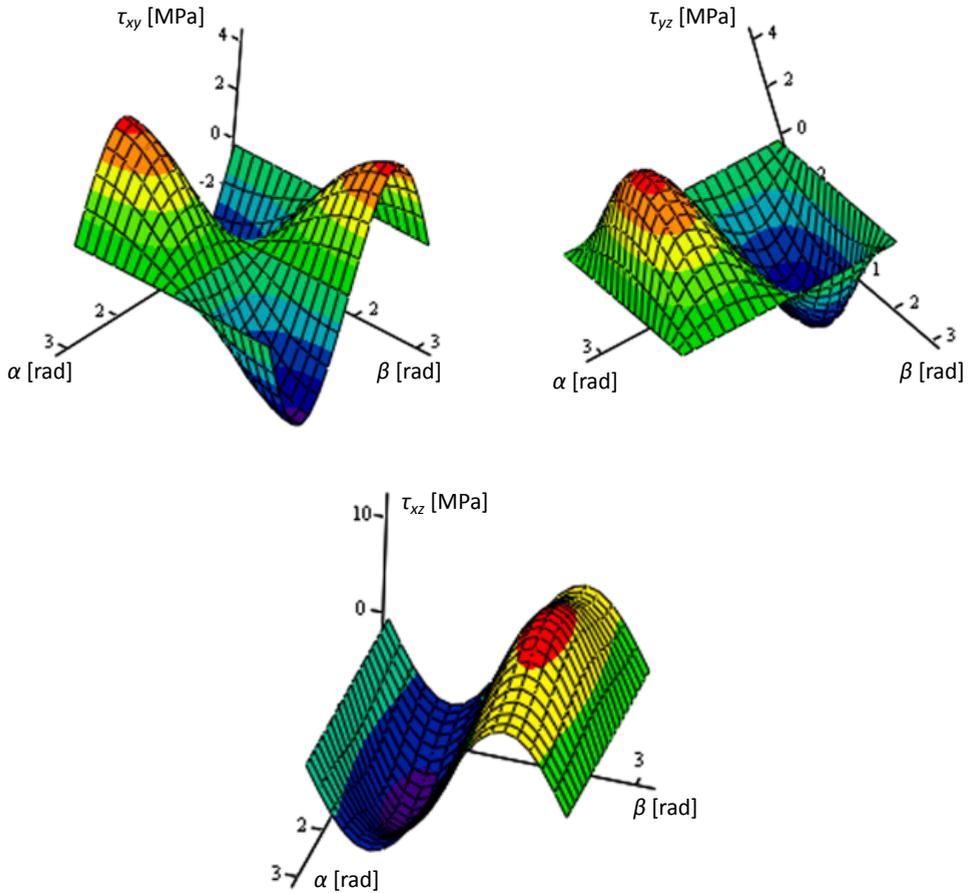
Fig. 3. Shear Stress vs. Wellbore Inclination and Azimuth graph
