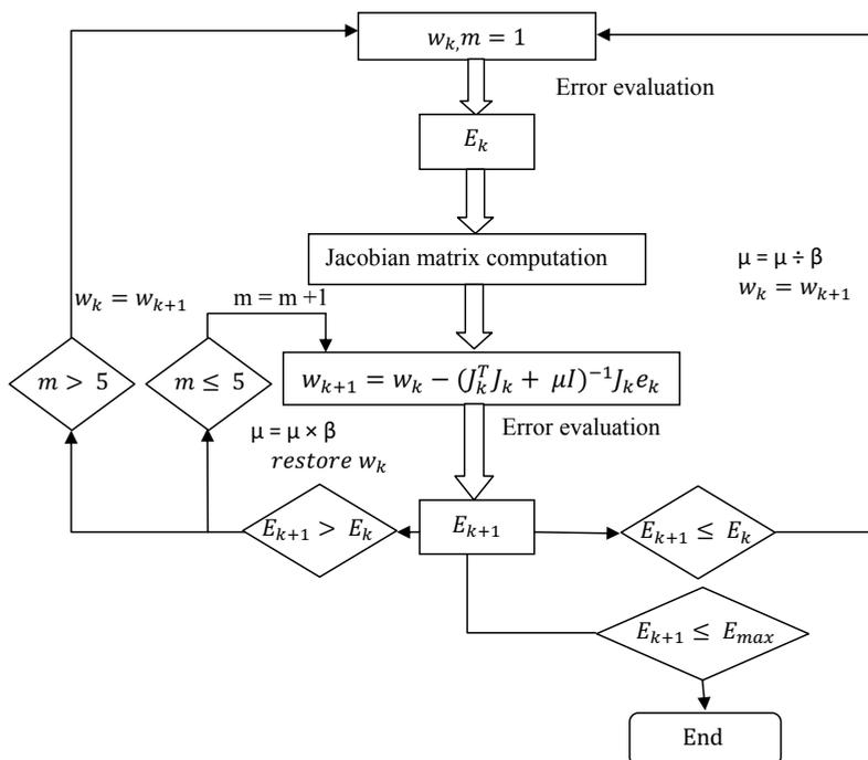
Fig. 2. Block diagram for training using Levenberg-Marquardt algorithm
