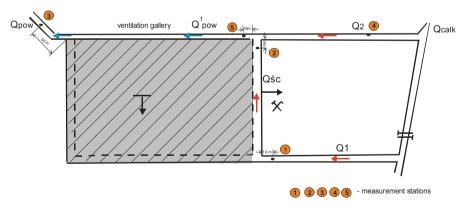
Fig. 5. Determination of ventilation methane content and the amount of methane emitted from goaves to workings during ventilation using "Y" method with a fresh air flow
