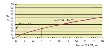
Fig. 2. Coal degassing degree  $\eta_s$  of the mined seam while being cut with a shearer depending on its methane content  $M_o$  (Krause, 2009)
