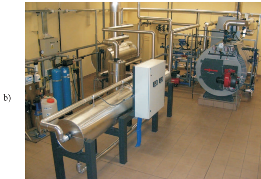
Figure 5. Experimental installation: a) main components of experimental facility: 1 – steam boiler, 2 – heat exchanger, 3 – deaerator, 4 – drain valve, 5 – steam header, 6 – orifice, P – pressure measuring device, T – thermometer; b) general view.
