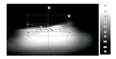
Fig. 14. The view of a light spot of low beam light reflector RE03411 (H4) together with indicated places of luminance measurement
