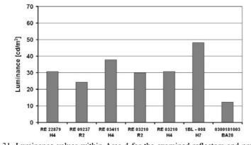
Fig. 31. Luminance values within Area 4 for the examined reflectors and projector
