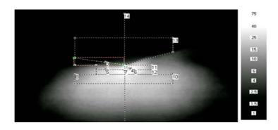
Fig. 10. The view of a light spot of low beam light reflector RE03210 (R2) together with indicated places of luminance measurement
