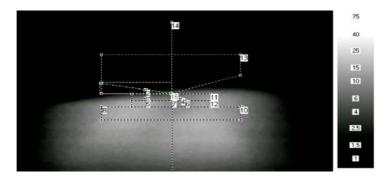
Fig. 6. The view of a light spot of low beam light reflector 0 -300-181-003 (BA20D) together with indicated places of luminance measurement
