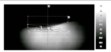
Fig. 8. The view of a light spot of low beam light reflector RE09237 (R2) together with indicated places of luminance measurement
