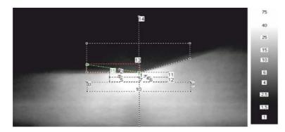
Fig. 4. The view of a light spot of low beam light projector 1BL-008 (H7) together with indicated places of luminance measurement
