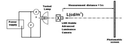
Fig. 2. Measurement station diagram
