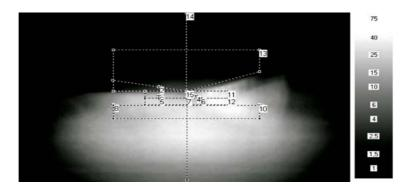
Fig. 12. The view of a light spot of low beam light reflector RE22879 (H4) together with indicated places of luminance measurement
