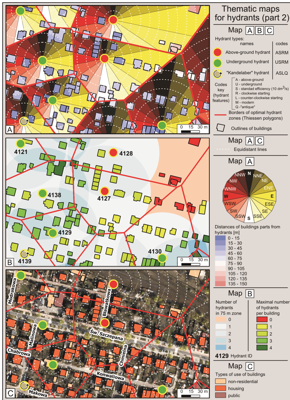
Fig. 4. Visualization of information about hydrants in relation to buildings and their types
