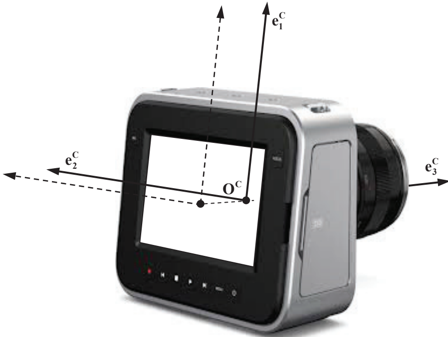
Fig. 2. The way of bonding the reference system \mathfrak{S}^C and the camera
