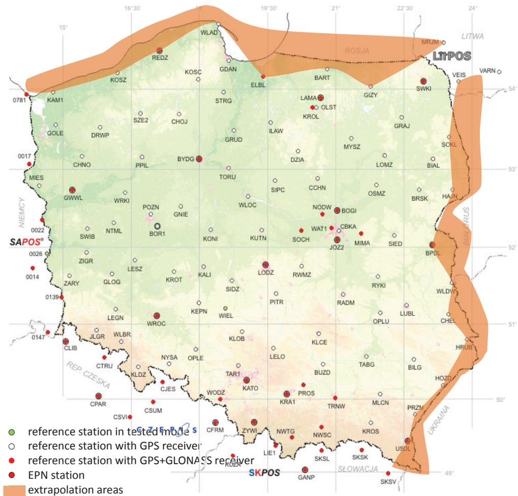
Fig. 1. ASG EUPOS system network and areas with correction extrapolation
