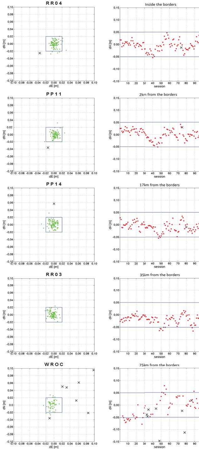
Fig. 3. Test sites' horizontal (left) and vertical (right) coordinate residuals obtained on 19 July 2012
