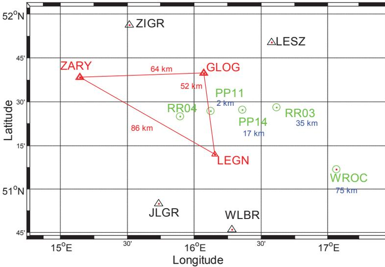
Fig. 2. Test network geometry (red – reference stations, green – test sites)
