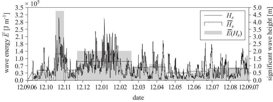
**Figure 8.** Hourly  $\overline{H}_s$  and time-averaged ( $\overline{H}_s$ ) significant wave heights together with wave energy  $\overline{E}$  averaged over time periods  $\Delta t_k$
