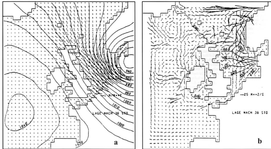
**Figure 14.** Extreme surge of the static type. Meteorological and oceanographic situation after a 36 h simulation; (a) pressure [HPa] and wind stress [ $\text{N m}^{-2}$ ], (b) water level [m] and transport [ $\text{m}^2 \text{s}^{-1}$ ]. From an unpublished thesis in the library of the University of Hamburg
