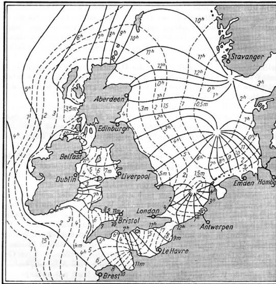
**Figure 2.** Co-phase lines (solid – hours) and co-range lines (dashed – metres) for the semidiurnal tides  $M_2 + S_2$ . From Sager (1959)
