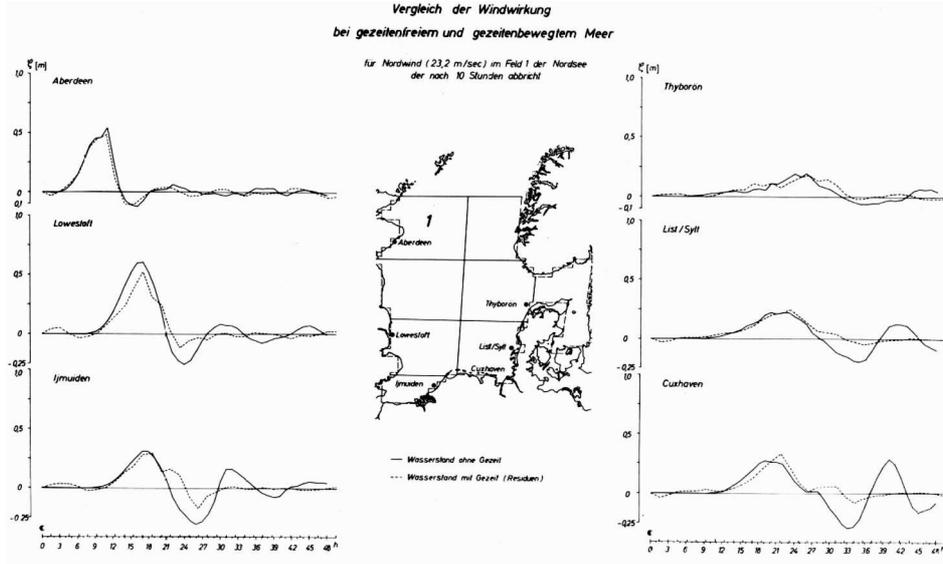
**Figure 10.** Propagation of a wind surge generated by a northerly wind of  $23.2 \text{ m s}^{-1}$  speed and 10 h duration in field 1. Solid line – water level without tidal interaction, dashed line – water level with tidal interaction. From Sündermann (1966)
