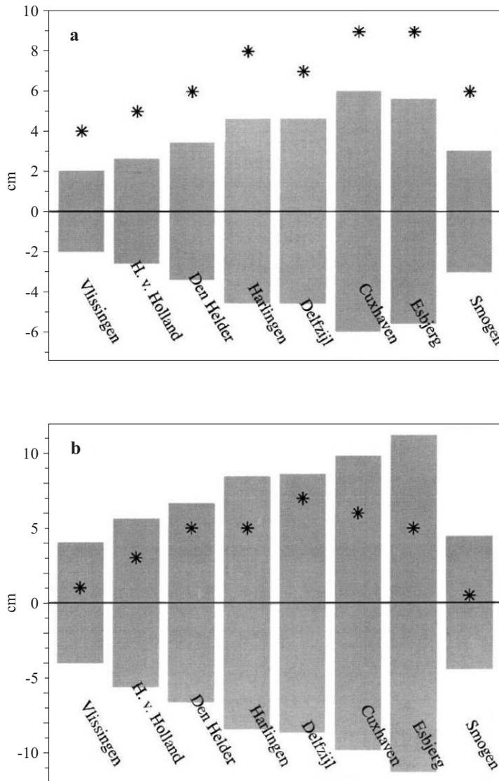
**Figure 19.** Differences in high water level for the period 1900–1996 ( $2 \times \text{CO}_2$  scenario – today, 5-winter-mean; asterisks). The estimated variability ( $\pm 2$  standard deviations) of all 5-winter-means is added in grey; (a) 50% percentile, (b) 90% percentile. From Langenberg et al. (1999)
