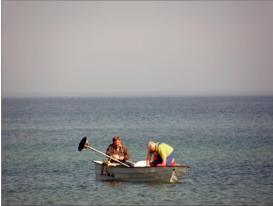
Figure 5. Seismo-acoustic measurements using the side-mounted StrataBox (the transducer pole, attached to the boat's side via an articulated joint, before being lowered to water) near CRS Lubiatowo in May 2009
