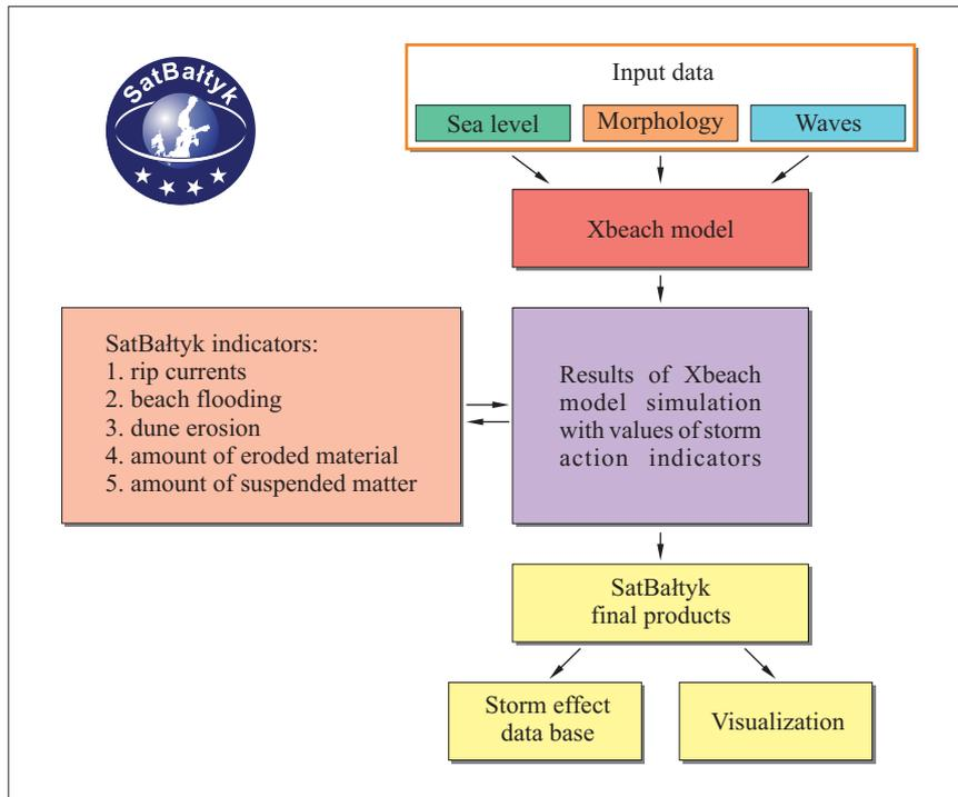
**Figure 11.** A scheme of the Xbeach system
